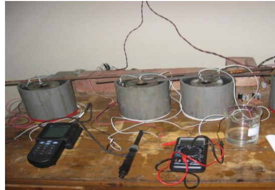
Fig. 7. Test setup for the determination of pH and charges passed in concrete.
