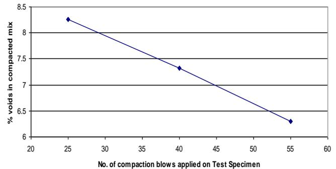
Fig. 3. Number of blows applied on the specimen v/s air voids
