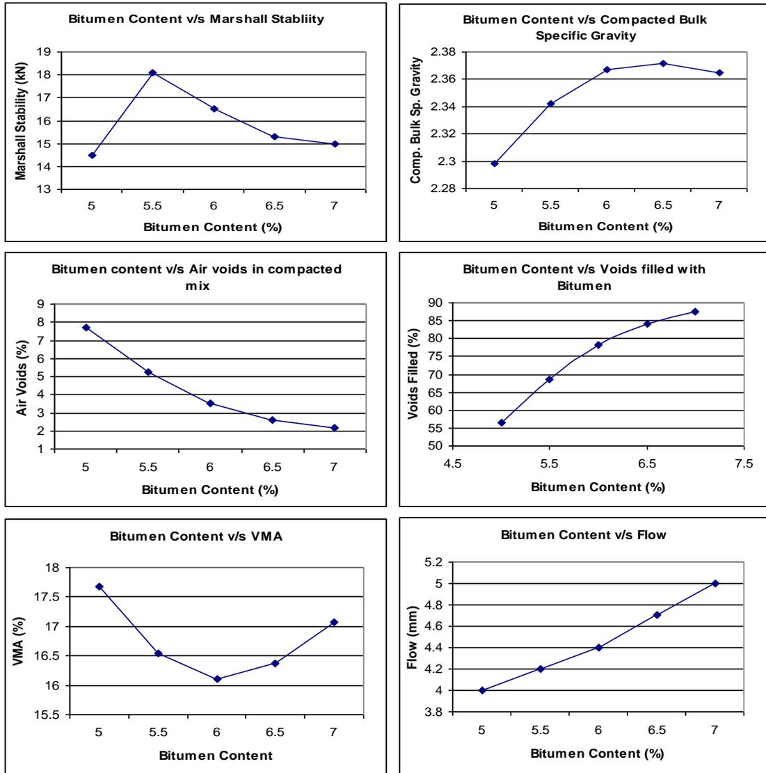
Fig. 1. Characteristics curves of AC mix properties
