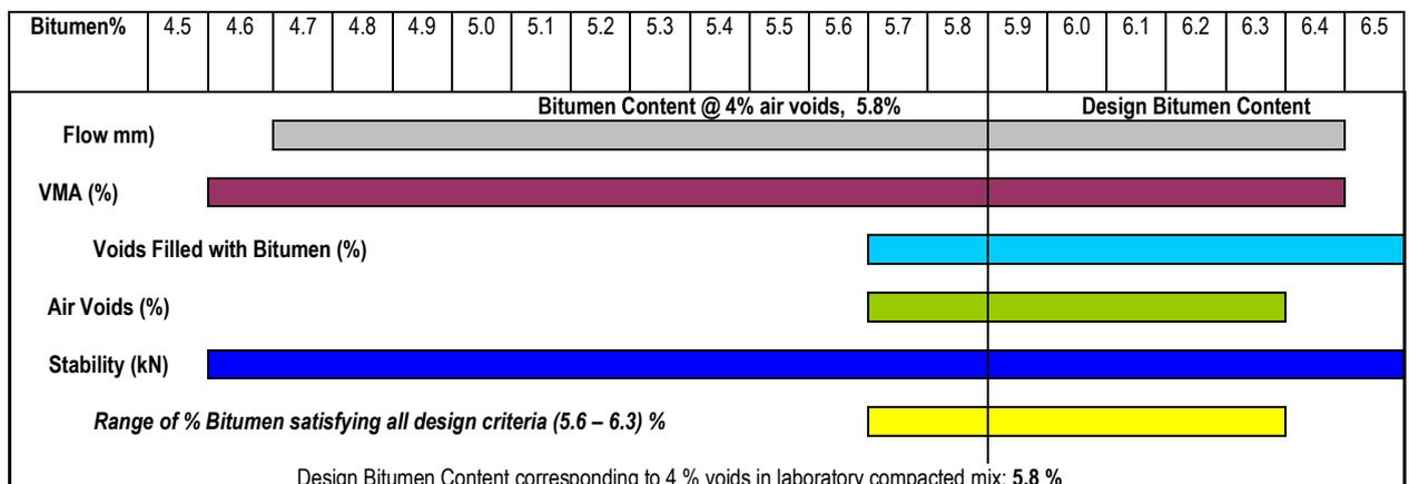
Fig. 2. Determination of design bitumen content for optimum mix
