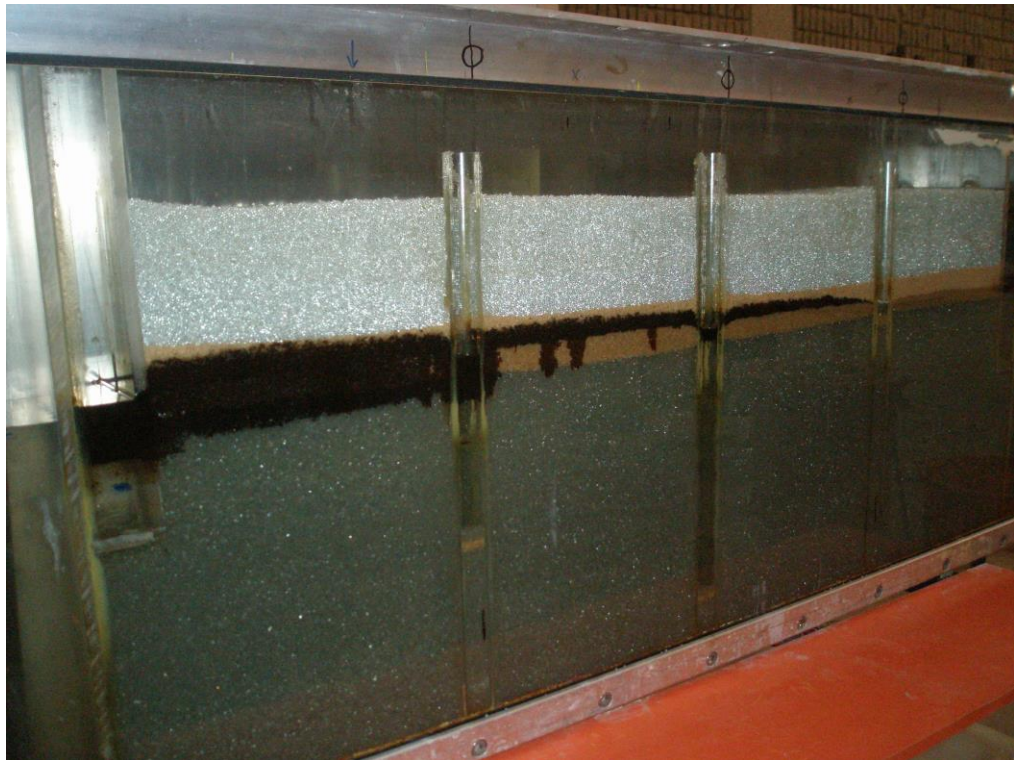
Fig. 3. Effect of heterogeneity on flow and distribution of LNAPL
