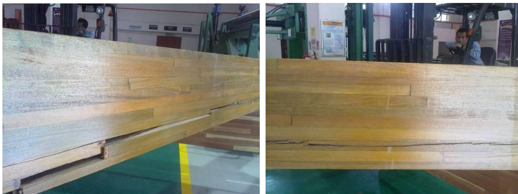
Fig. 5. Failure of Resak beams showing similar pattern as Keruing, failed in timber
