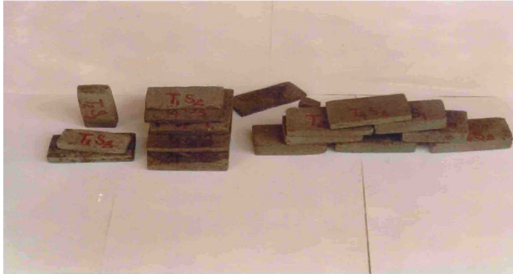
Figure 3 Kenaf brake pad samples
