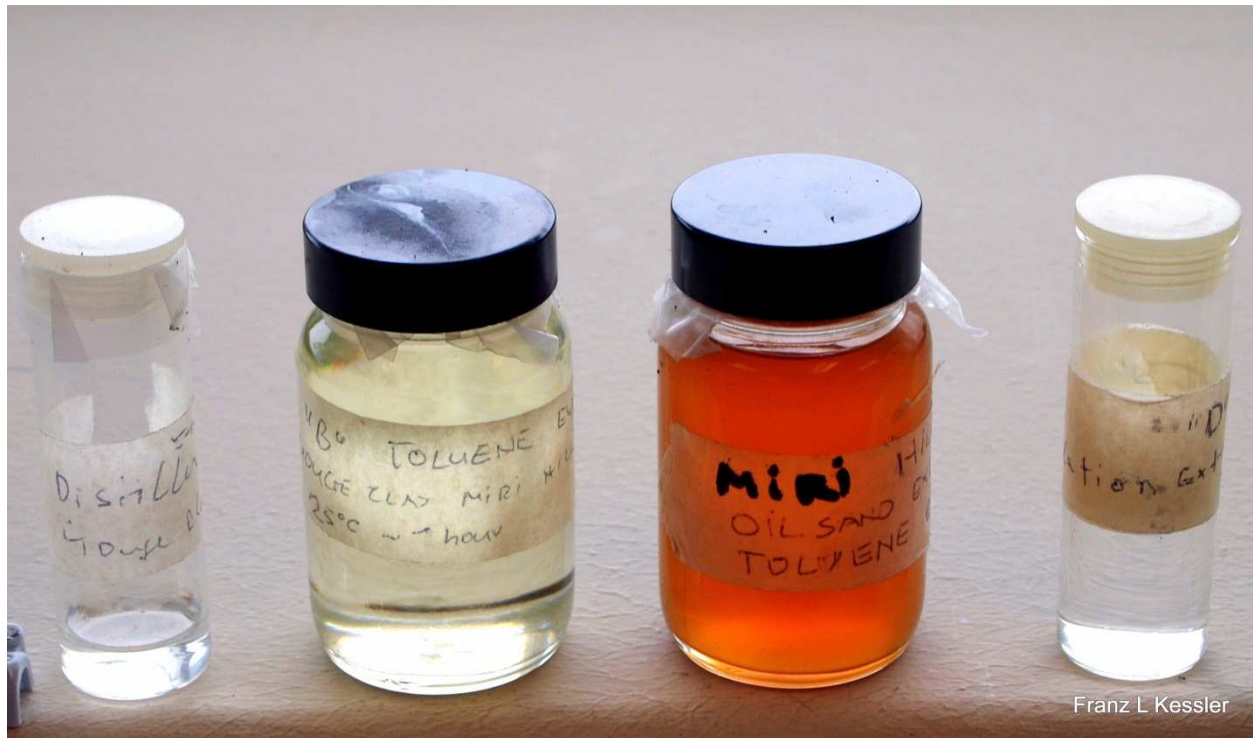
Fig. 6: Extractions from oil sands of sample area 2. Two different sand layers containing hydrocarbons were extracted using Toluene. Note the colour difference between the two bottles in the center: faint yellow and dark orange. The latter belongs to a vertical steepened oil sand outcrop, of very strong petroleum smell and sealed by an overthrust fault (shown in Fig. 4). The estimated oil saturation in this sand may be in the order of 20 %. The bottles on either side contain distillate from the oil sands (please note the clear colour, there is little or no oil present in the distillates).
