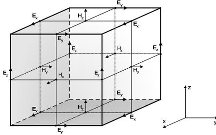
FIGURE 1. An FDTD cell or Yee cell showing the positions of electric and magnetic field components
