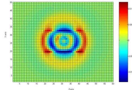
FIGURE 3. Electromagnetic propagation from PIFA using FDTD
