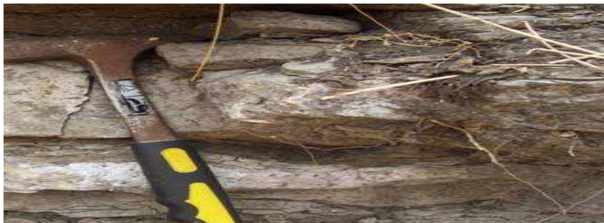
FIG 1: Nodular-marl and shale intercalation in the New Netim Marl
