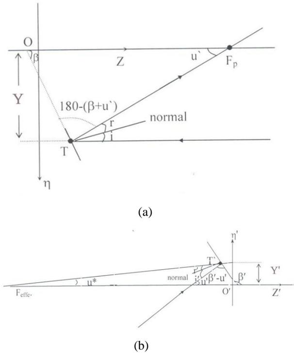
Fig. 2. Ray reflection at the Gregorian mirrors. (a) Ray behavior at the Gregorian primary Mp . (b) Reflection at the secondary Gregorian mirror Ms.
