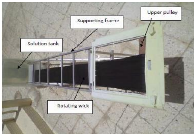
Fig. 8. View of the experimental Rotating desiccant wick.
