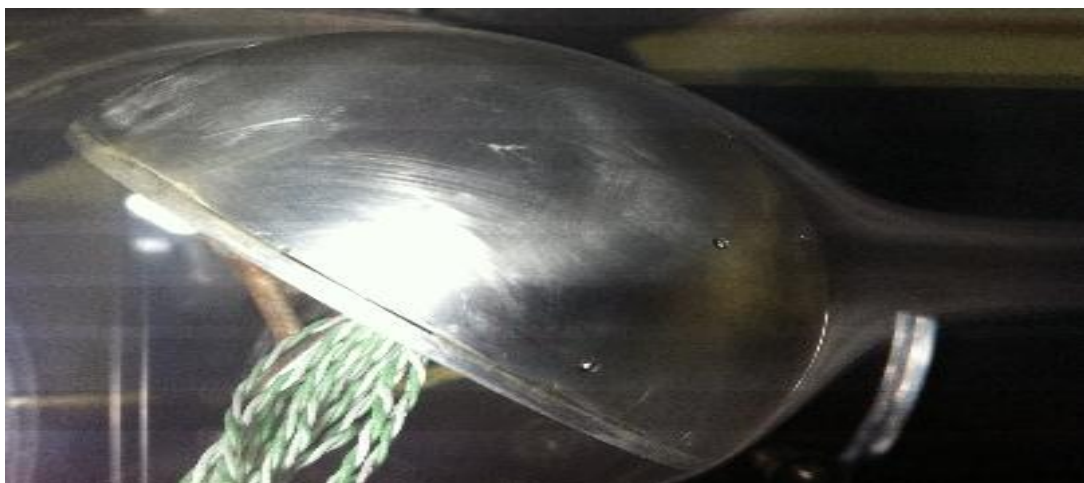
Fig. 9. Smoke generated flow around hemisphere showing separation flow on the trailing surface, Re = 2.5E^{+05}
