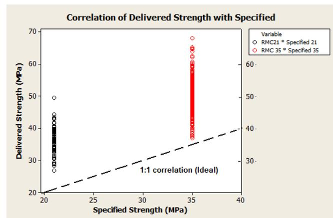
Fig. 3. Correlation of Delivered Compressive Strength with the Specified Value for the Ready-Mixed Concrete Production Plant
