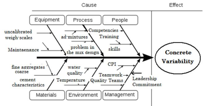
Fig. 8. Ishikawa Diagram for Root Causes Analysis of Concrete Variability
