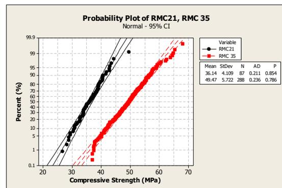
Fig. 5. Probability Plot of the Concrete Production Plant
