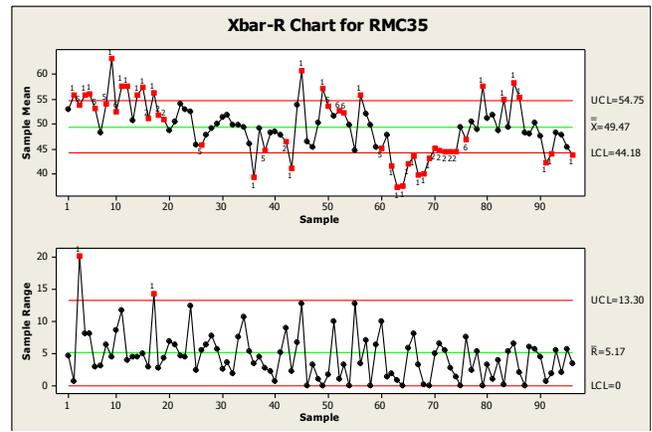
Fig. 6.  $\bar{X}$ -R Control Charts for Ready-Mixed Concrete (M35)
