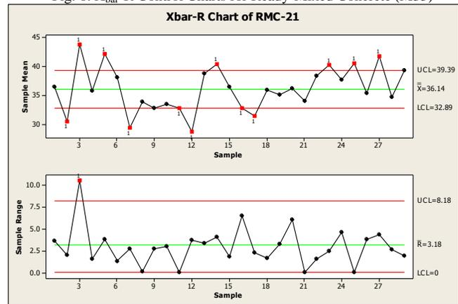
Fig. 7.  $\bar{X}$ -R Control Charts for Ready-Mixed Concrete (M21)
