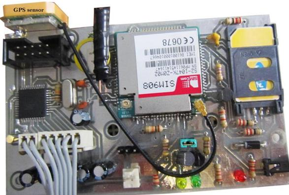
Fig. 9. experimental sample of micro board and GPRS
