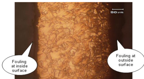
Fig. 3.4. Metallographic test results obtained from sampling point 3 (Etching: 2gr K 2 Cr 2 O 7 + 8 ml H 2 SO 4 + 4 ml saturated NaCl _100 ml H 2 O).
