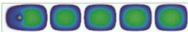
Fig. 2. a E-Field pattern in the XY plane cut through empty shorted rectangular waveguide section
