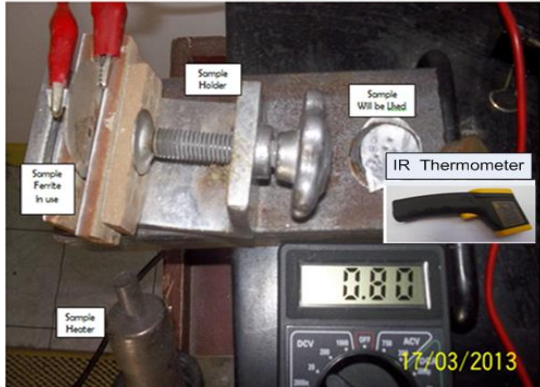
Fig. 15. Network of the simple measurement instrumentation Of The thermoelectric Power .
