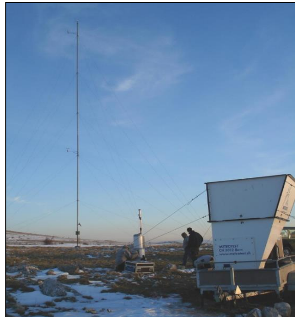
Fig. 3. Measuring mast, SODAR and LIDAR at the location of Mali grad – Mostar.
