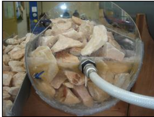
Fig. 3. Armouring due to iron precipitation in open limestone channel
