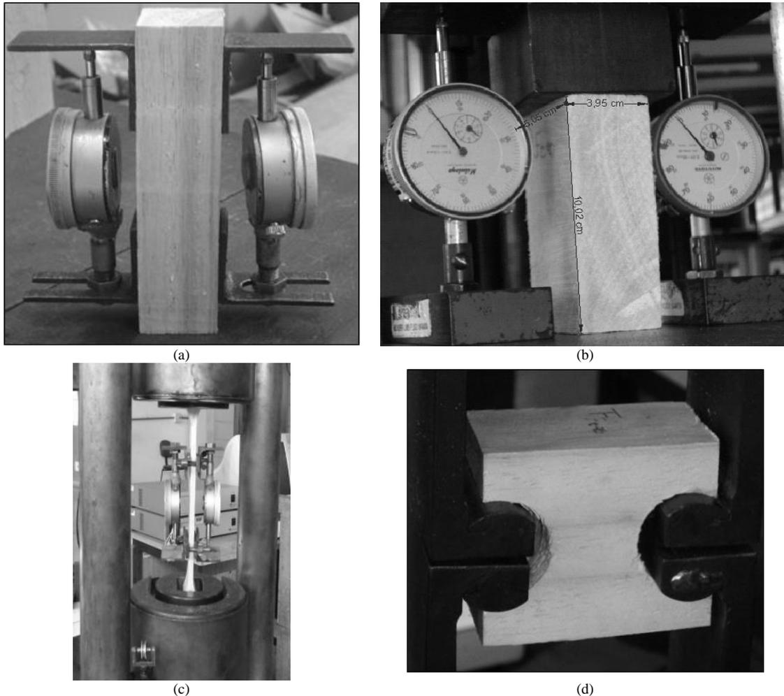
Fig. 1. Instrumented specimens for (a) parallel to grain compression, (b) perpendicular to grain compression, (c) parallel to grain tension and (d) perpendicular to grain tension.
