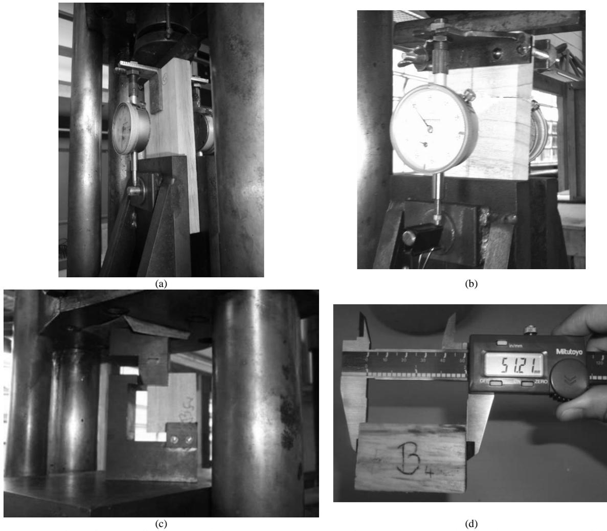
Fig. 2. Instrumented specimens for (a) parallel to grain embedment, (b) perpendicular to grain embedment, (c) parallel to grain shear and (d) specific gravity tests.
