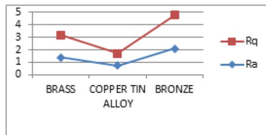
Fig. 3.6 Surface Roughness Values (Before Machining)
