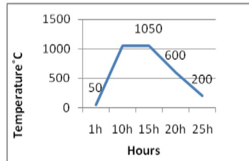
Fig 2.2.1 Oven Temperature Distribution
