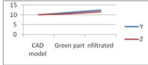
From the measured values it noticed that the variation in y direction is high compared to other two directions x and z. The effect of type of infiltrants has not much affected the dimensions.
