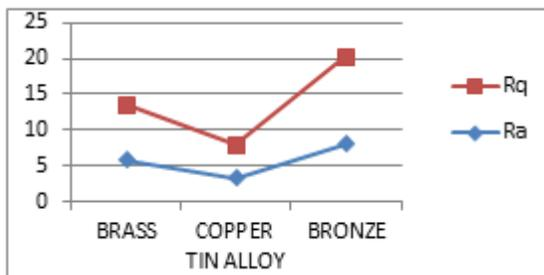
Fig. 3.7 Comparison of Surface Roughness Values (After Machining)
