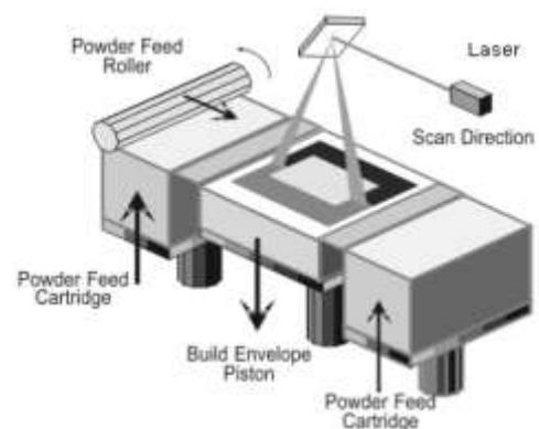
Fig. 1.1 sinterstation 2500<sup>plus</sup> machine and its schematic
