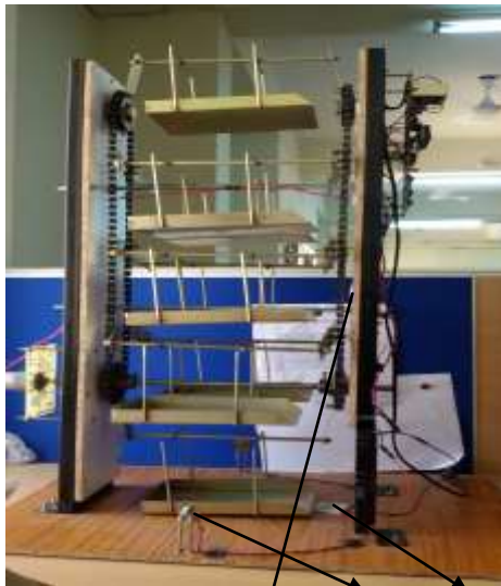
Fig. 2. Total structure With IR , PIEZO sensor &Magnetic switches
