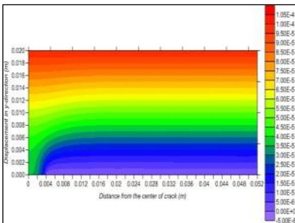
Fig. 19. Contour of Displacement in Y-Direction Calculating by MFree Method When the Fiber Volume Fraction is (37.5%) and Crack Length is (0.008 m).
