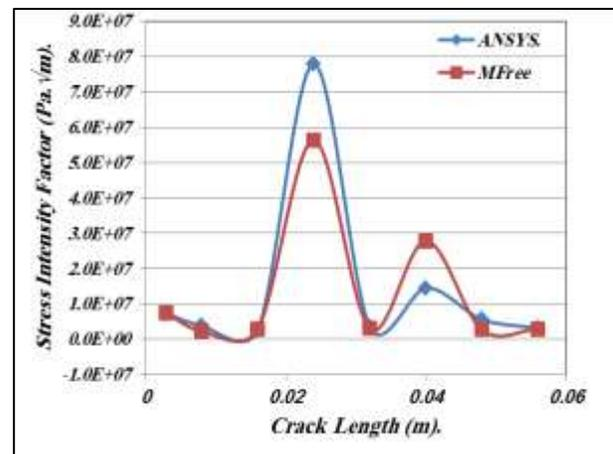
Fig. 4. Variation of Stress Intensity Factor with the Increasing of Crack Length When Volume Fraction of Fiber is (26%).
