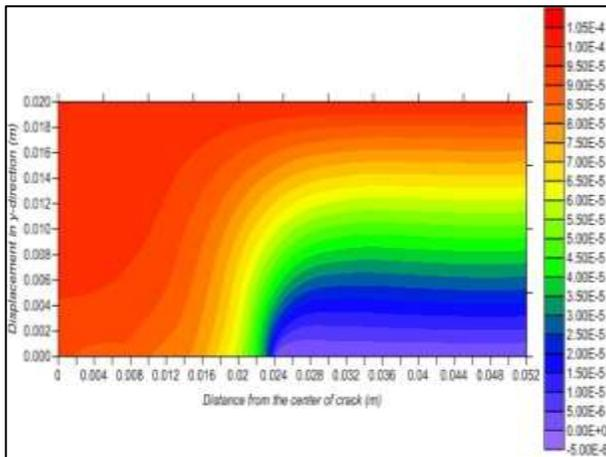
Fig. 29. Contour of Displacement in Y-Direction Calculating by MFree Method When the Fiber Volume Fraction is (37.5%) and Crack Length is (0.048 m).
