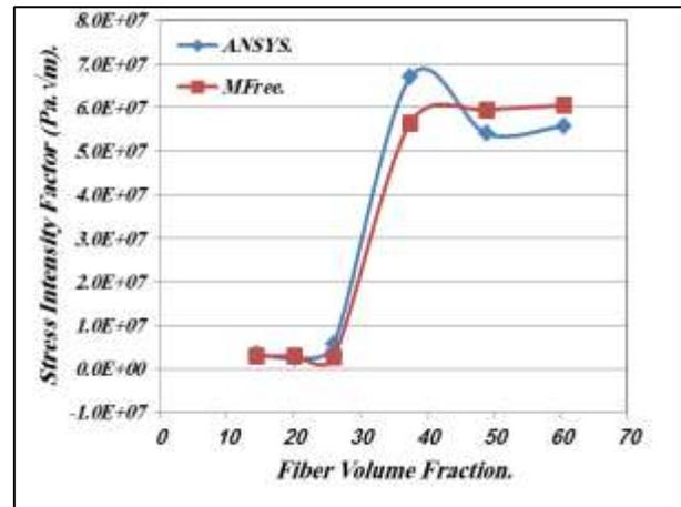
Fig. 14. Variation of Stress Intensity Factor with the Increasing of Fiber Volume Fraction When Crack Length is (0.048 m).
