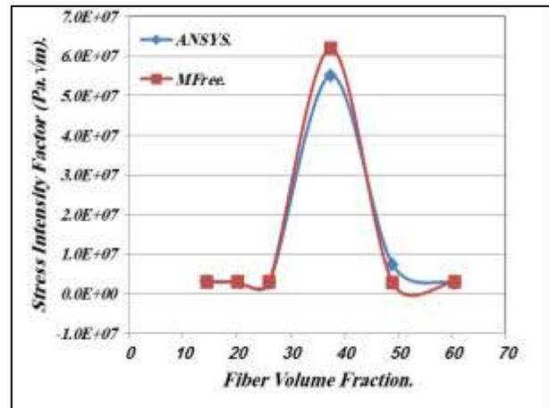
Fig. 10. Variation of Stress Intensity Factor with the Increasing of Fiber Volume Fraction When Crack Length is (0.016 m).
