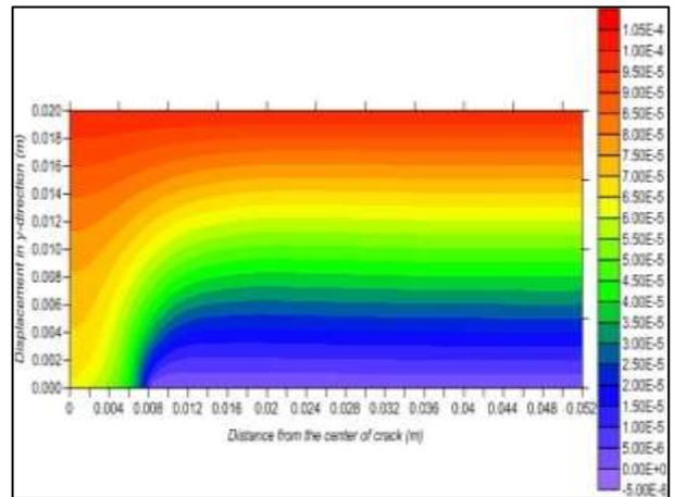
Fig. 21. Contour of Displacement in Y-Direction Calculating by MFree Method When the Fiber Volume Fraction is (37.5%) and Crack Length is (0.016 m).
