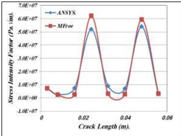
Fig. 6. Variation of Stress Intensity Factor with the Increasing of Crack Length When Volume Fraction of Fiber is (49%).
