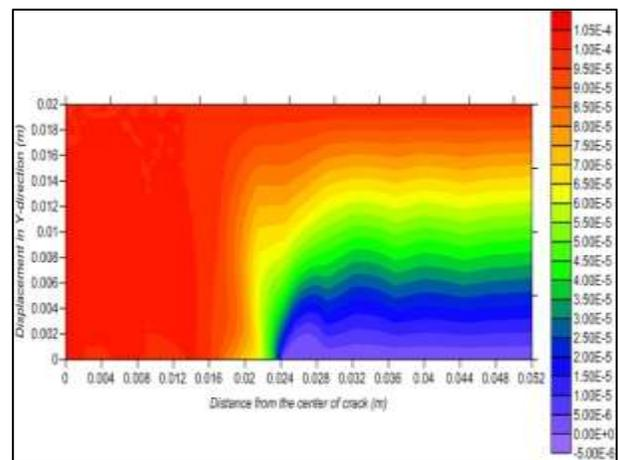
Fig. 28. Contour of Displacement in Y-Direction Calculating by FEM When the Fiber Volume Fraction is (37.5%) and Crack Length is (0.048 m).
