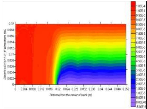
Fig. 25. Contour of Displacement in Y-Direction Calculating by FEM When the Fiber Volume Fraction is (37.5%) and Crack Length is (0.04 m).
