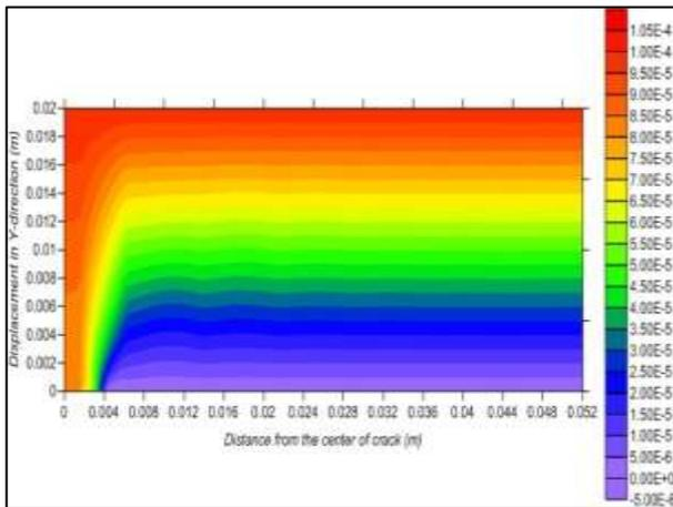
Fig. 18. Contour of Displacement in Y-Direction Calculating by FEM When the Fiber Volume Fraction is (37.5%) and Crack Length is (0.008 m).
