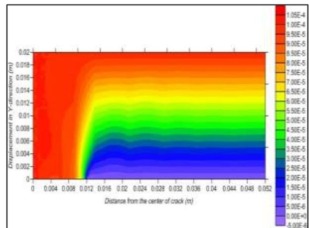
Fig. 22. Contour of Displacement in Y-Direction Calculating by FEM When the Fiber Volume Fraction is (37.5%) and Crack Length is (0.024 m).
