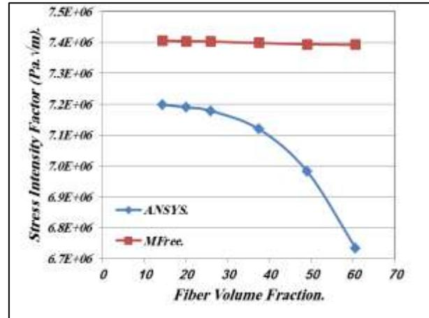
Fig. 8. Variation of Stress Intensity Factor with the Increasing of Fiber Volume Fraction When Crack Length is (0.003 m).
