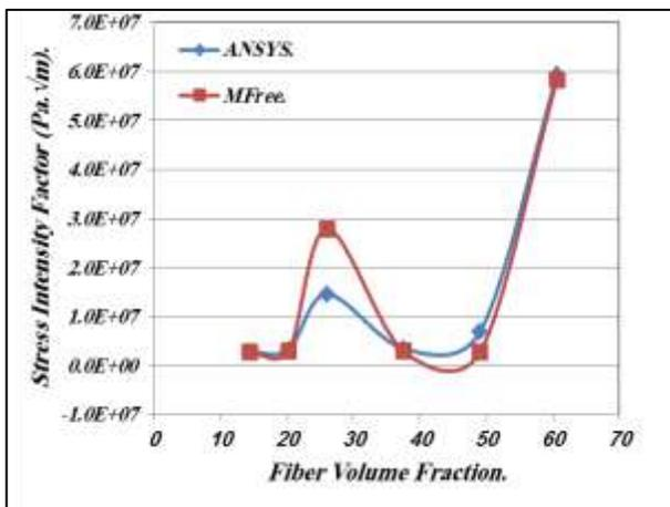
Fig. 13. Variation of Stress Intensity Factor with the Increasing of Fiber Volume Fraction When Crack Length is (0.040 m).
