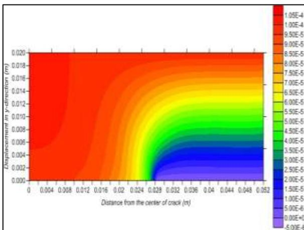
Fig. 31. Contour of Displacement in Y-Direction Calculating by MFree Method When the Fiber Volume Fraction is (37.5%) and Crack Length is (0.056 m).
