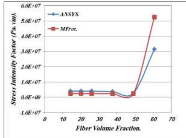
Fig. 9. Variation of Stress Intensity Factor with the Increasing of Fiber Volume Fraction When Crack Length is (0.008 m).
