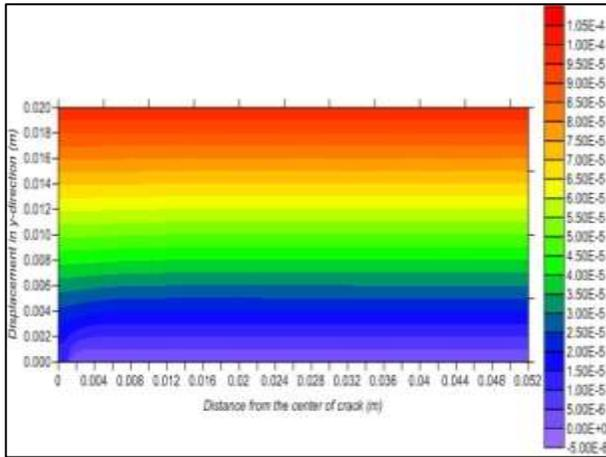
Fig. 17. Contour of Displacement in Y-Direction Calculating by MFree Method When the Fiber Volume Fraction is (37.5%) and Crack Length is (0.003 m).
