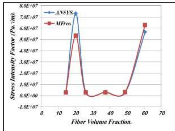
Fig. 15. Variation of Stress Intensity Factor with the Increasing of Fiber Volume Fraction When Crack Length is (0.056 m).
