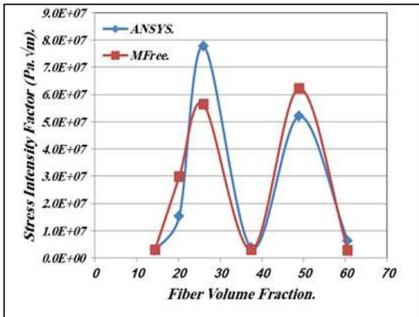
Fig. 11. Variation of Stress Intensity Factor with the Increasing of Fiber Volume Fraction When Crack Length is (0.024 m).
