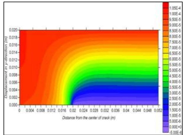
Fig. 27. Contour of Displacement in Y-Direction Calculating by MFree Method When the Fiber Volume Fraction is (37.5%) and Crack Length is (0.04 m).
