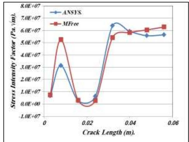
Fig. 7. Variation of Stress Intensity Factor with the Increasing of Crack Length When Volume Fraction of Fiber is (60.6%).
