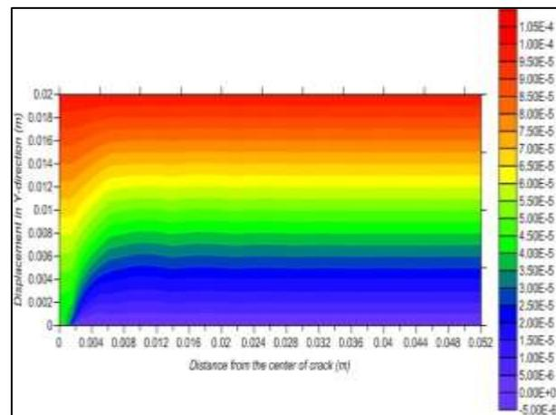
Fig. 16. Contour of Displacement in Y-Direction Calculating by FEM When the Fiber Volume Fraction is (37.5%) and Crack Length is (0.003 m).
