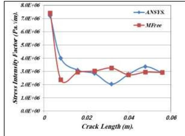
Fig. 2. Variation of Stress Intensity Factor with the Increasing of Crack Length When Volume Fraction of Fiber is (14.4%).
