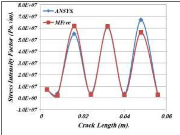
Fig. 5. Variation of Stress Intensity Factor with the Increasing of Crack Length When Volume Fraction of Fiber is (37.5%).
