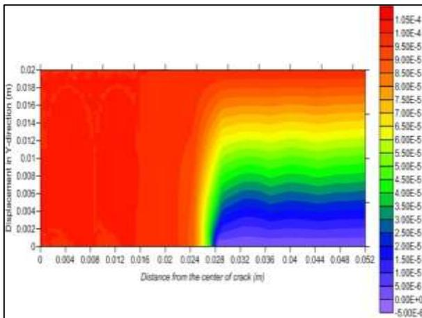
Fig. 30. Contour of Displacement in Y-Direction Calculating by FEM When the Fiber Volume Fraction is (37.5%) and Crack Length is (0.056 m).
