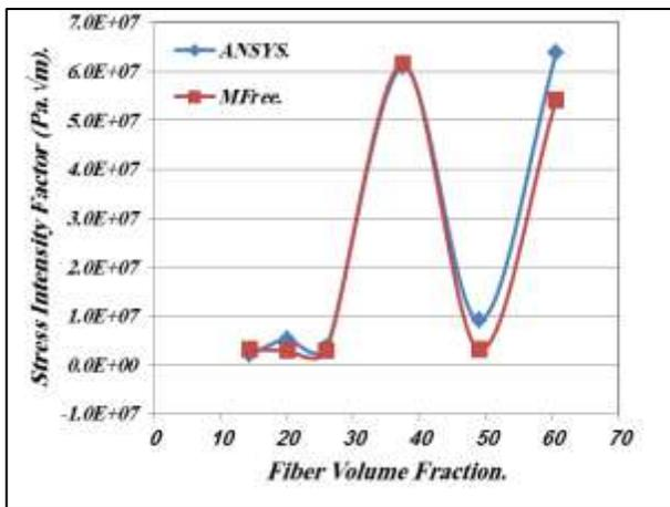
Fig. 12. Variation of Stress Intensity Factor with the Increasing of Fiber Volume Fraction When Crack Length is (0.032 m).
