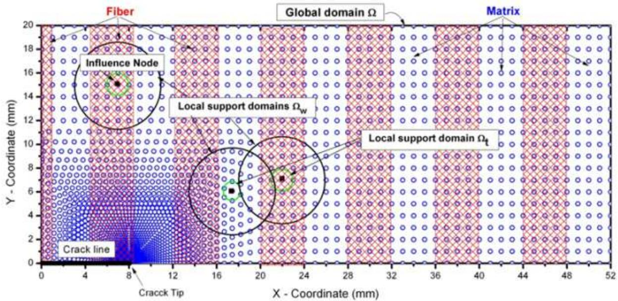
Fig. (1-a). MFree Modeling for Composite Material ( The Nodal Distribution for the Global Domain)[22,29]
