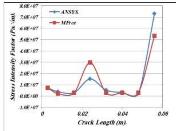
Fig. 3. Variation of Stress Intensity Factor with the Increasing of Crack Length When Volume Fraction of Fiber is (20.2%).
