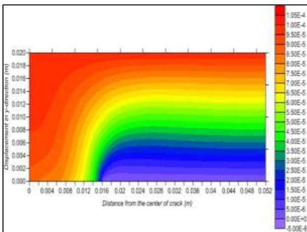
Fig. 25. Contour of Displacement in Y-Direction Calculating by MFree Method When the Fiber Volume Fraction is (37.5%) and Crack Length is (0.032 m).
