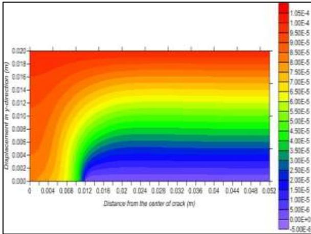
Fig. 23. Contour of Displacement in Y-Direction Calculating by MFree Method When the Fiber Volume Fraction is (37.5%) and Crack Length is (0.024 m).
