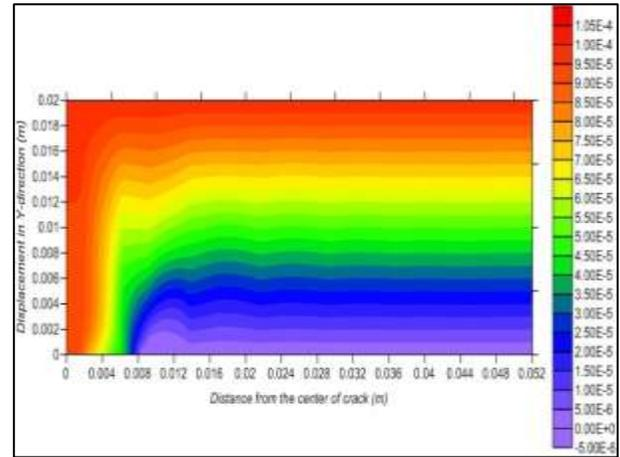
Fig. 20. Contour of Displacement in Y-Direction Calculating by FEM When the Fiber Volume Fraction is (37.5%) and Crack Length is (0.016 m).
