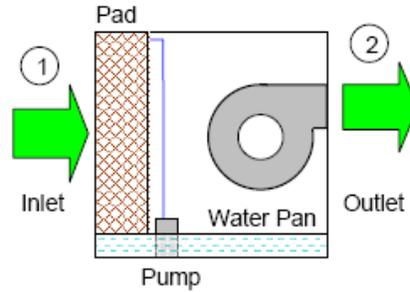
Fig. 1. Direct evaporative cooler
