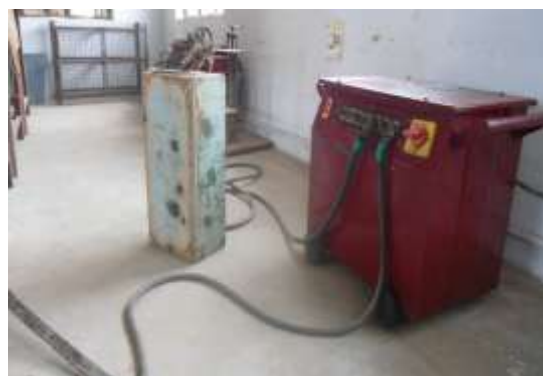
Fig.2. Experimental set up for SMAW process
