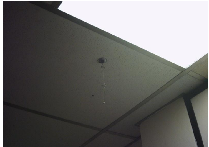
Fig. 3. Magnetically-Mounted Omni Antenna (2.4 GHz, 5 dBi)
