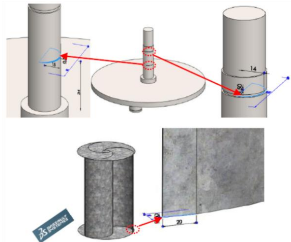
Fig. 3. Cracks growths settings
