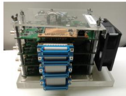
(b) A DPM box, consisting of a set of 4 DPMs (1 master and 3 slaves).
