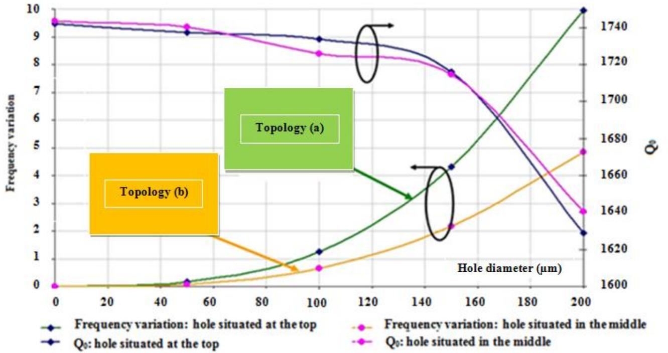
Fig. 3. variations of the frequency and the quality factor according to the whole diameter in two different cases.
