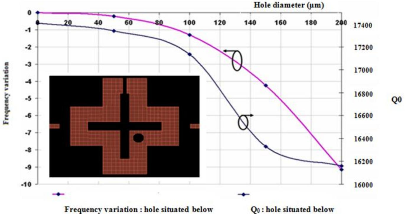
Fig. 6. variations of the frequency and the quality factor according to the hole diameter in the case of hole situated in the lower branch
