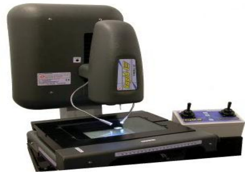
Fig. 4. Rapid – I Vision Measuring System (V 2015J LX) Model
