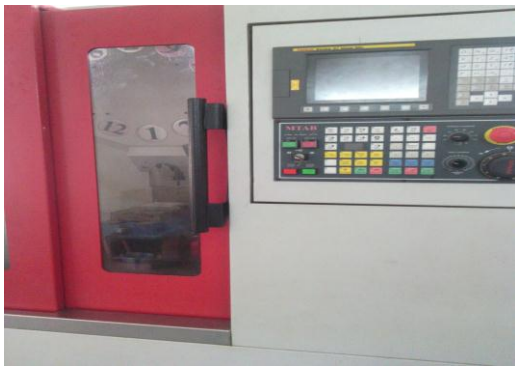
Fig. 2. CNC Vertical Machine Centre
