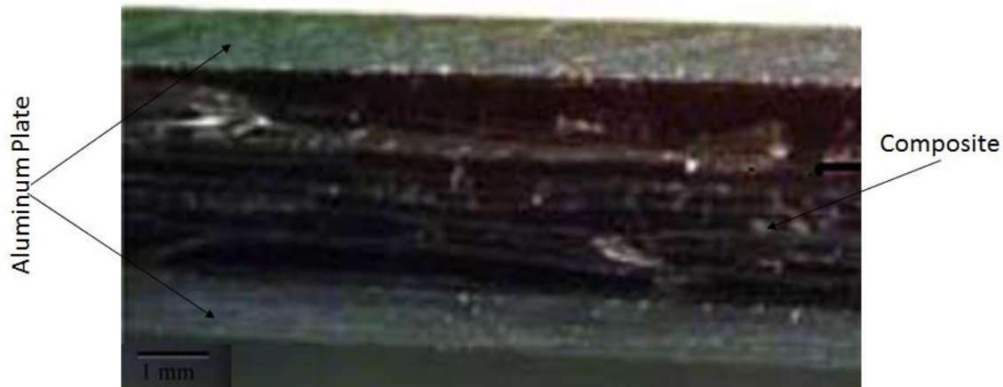
Fig. 1. GLARE specimen cross section
