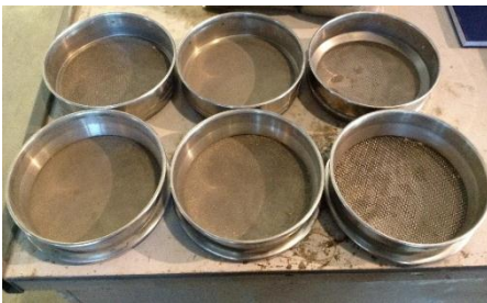
Fig. 1. Sieve containers of different mesh sizes are used for soil characterization.
