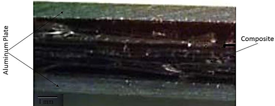
Fig. 1. GLARE specimen cross section [10]
