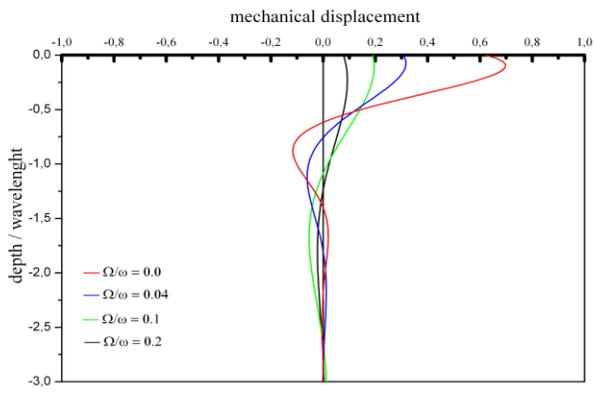
Fig. 10. Variation of  $x_1$  normalized components of mechanical displacement vs. depth (in wave-lengths) for different rotation ratios ( $\Omega/\omega$ ).
