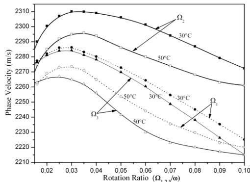
Fig.6. Variation of RW phase velocity vs. Large ratios ( $\Omega_{1,2,3}/\omega$ ) about three axis for the initial temperatures 30°C and 50°C, electroded surface and including centrifugal forces.
