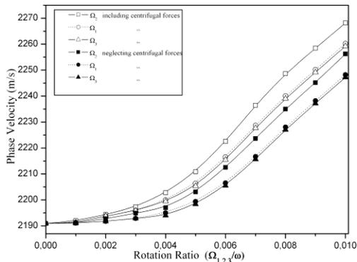
Fig.3. Variation of RW phase velocity vs. Small ratios ( $\Omega_{1,2,3}/\omega$ ) for electroded surface and the three axis with including/neglecting centrifugal forces.
