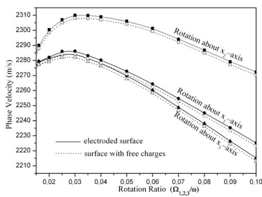
Fig. 8. Variation of RW phase velocity vs. Large ratios ( $\Omega_{1,2,3}/\omega$ ) about three axis for electroded/free charges surface with including centrifugal forces.
