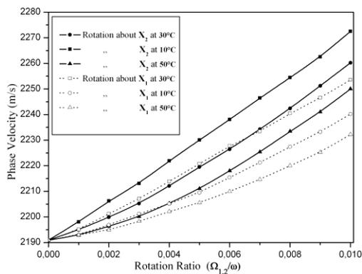
Fig.5. Variation of RW phase velocity vs. Small ratios ( $\Omega_{1,2}/\omega$ ) about the  $x_1$  and  $x_2$  axis for different initial temperatures with electroded surface.
