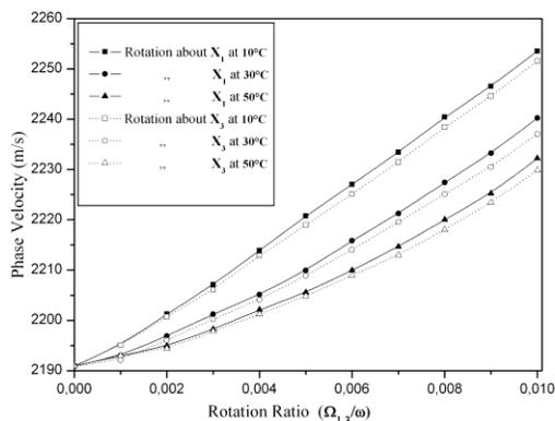
Fig.4. Variation of RW phase velocity vs. Small ratios ( $\Omega_{1,3}/\omega$ ) about the  $x_1$  and  $x_2$  axis for different initial temperatures with electroded surface.
