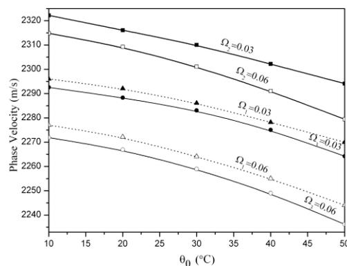
Fig.7. Variation of RW phase velocity vs. Preheating temperatures of the body ( $\theta_0$ ) about three axis with ratios ( $\Omega_{1,2,3}/\omega$ ) and electroded surface.
