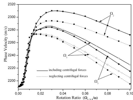
Fig. 2. Variation of RW phase velocity vs. Large rotation ratios ( $\Omega_{1,2,3}/\omega$ ) about three axis with electroded surface and including/neglecting centrifugal forces.
