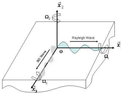
Fig.1. Rayleigh and BG waves propagation on  $x_2$  rotating thermopiezoelectric half space.
