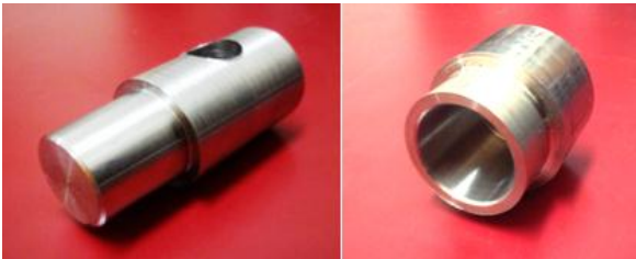
Fig. 2. Shaft and hub of implant sample
