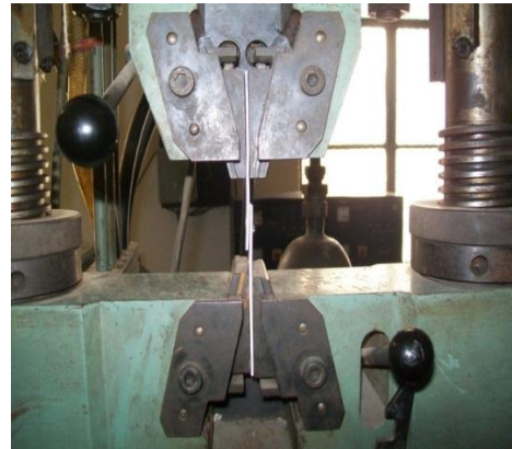
Fig. 3. Showing conducting of the tensile shear testing on universal testing machine.
