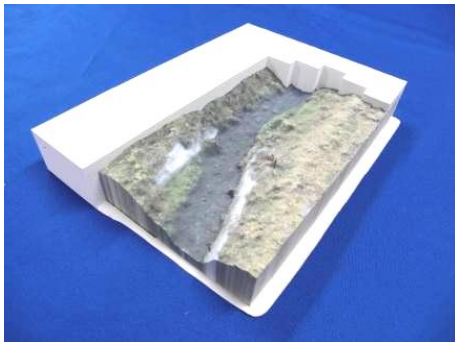
Fig. 15. 3D map model inside 337 pages of A4 size papers built by using the static photo images of the environment around the river
