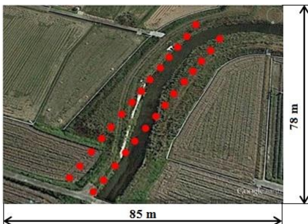
Fig. 3. Positions where static photo images and video images were captured by the fisheye-lens camera mounted on the multi-rotor drone
