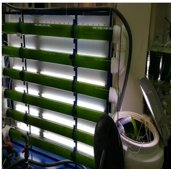
Fig. 1. Photo bioreactor for growing Scenedesmus .
