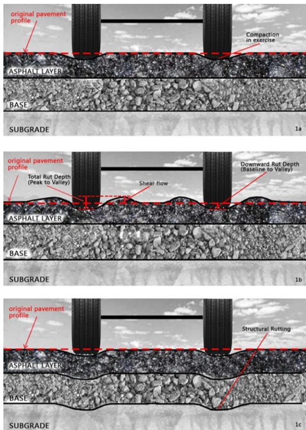
Fig. 1. Qualitative representation of different types of rutting.
