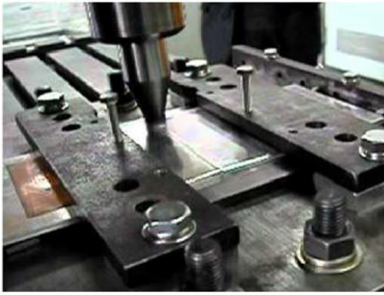
Fig. 2. Joining of alloys by FSW process
