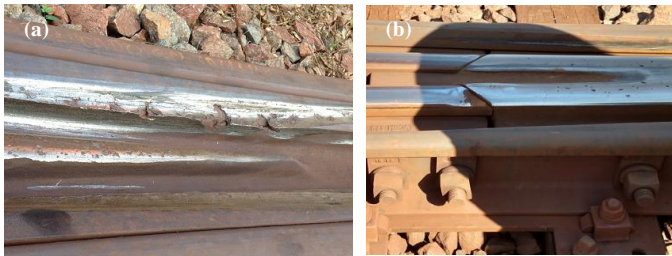
Fig. 3. Frog defects (a) severe superficial frog defect; (b) step between manganese and carbon steel in a frog heel.
