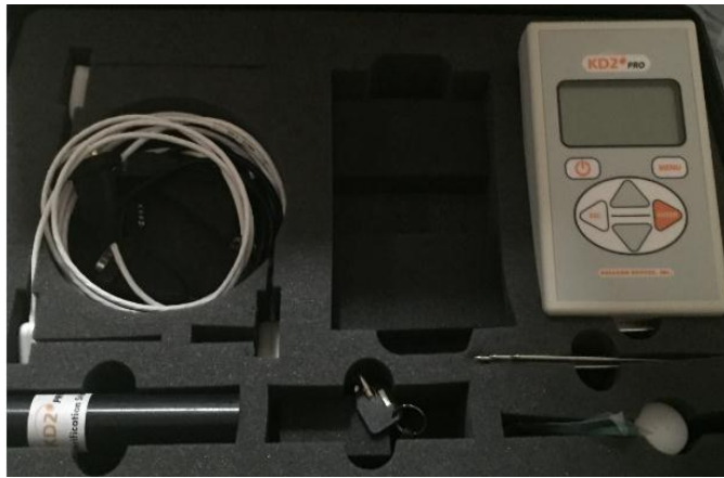
Fig. 1. Thermal conductivity measuring device
