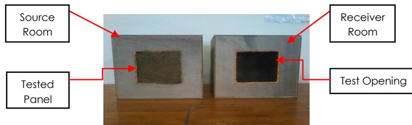
Fig. 14. Placement of the tested panel.
