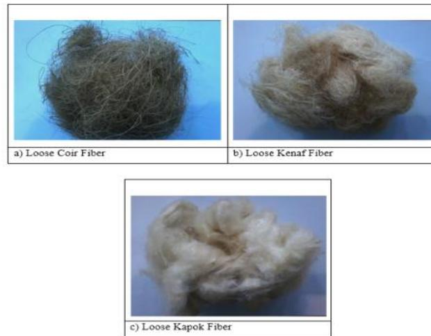
Fig. 8. Loose forms: (a) Coir Fiber (b) Kenaf Fiber (c) Kapok Fiber.
