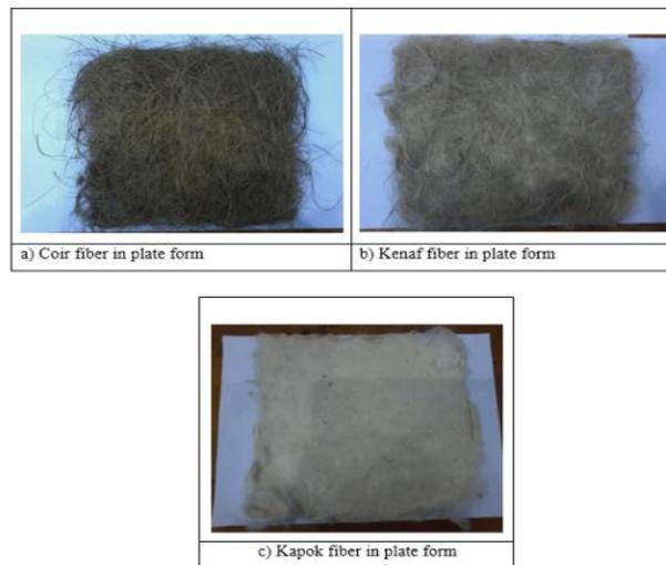
Fig. 10. Fibers in plate forms: (a) Coir Fiber (b) Kenaf Fiber (c) Kapok Fiber
