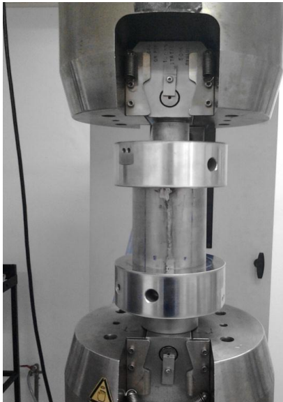
Fig. 4. Compression test arrangements of cylindrical model C1.
