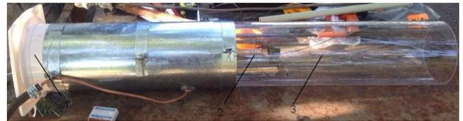
Fig. 1b. General view of the experimental setup. 1 - the air supply system, 2 - V-gutter flameholders, 3 - the quartz tube
