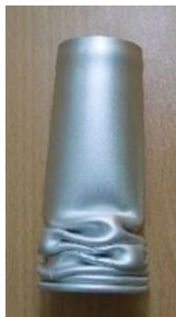
Fig. 3. Mixed mode deformation pattern for virgin tube by Yob et al.[13].
