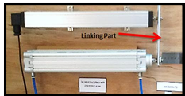
Fig. 4. The Pneumatic Cylinder and Linear Position Sensor
