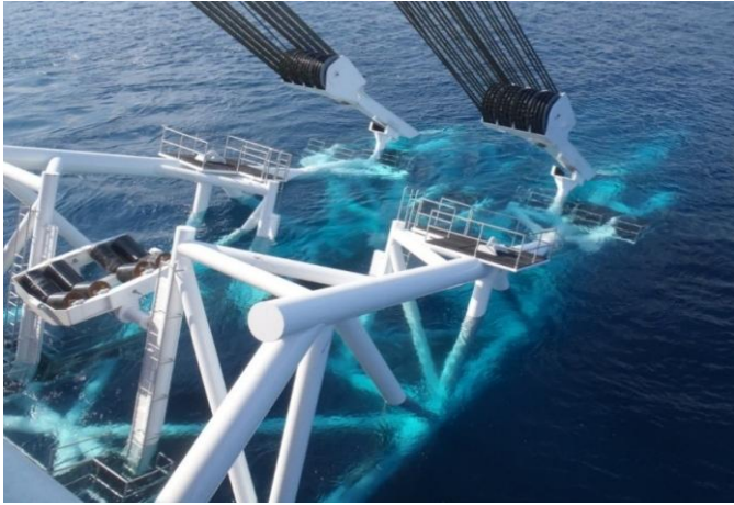
Fig. 2. Stinger; usual space frame tubular structure [2]
