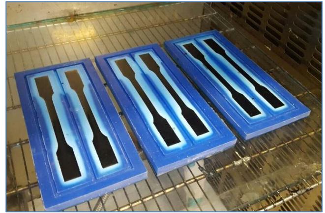
Fig. 3. Silicon moulds used for casting the tensile specimens
