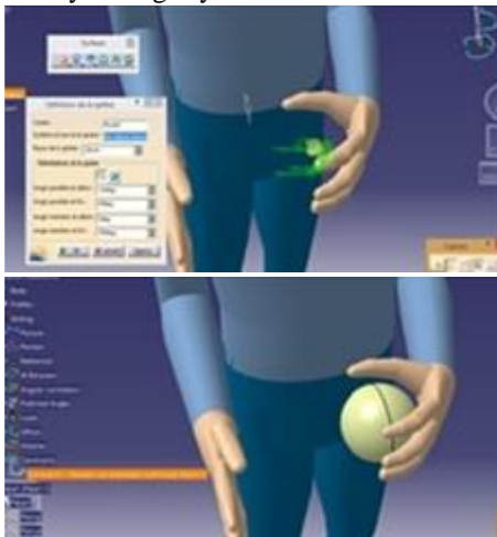
Fig. 11. Selection of the hand with spherical posture via 'Catia's 'Human Builder' module.
