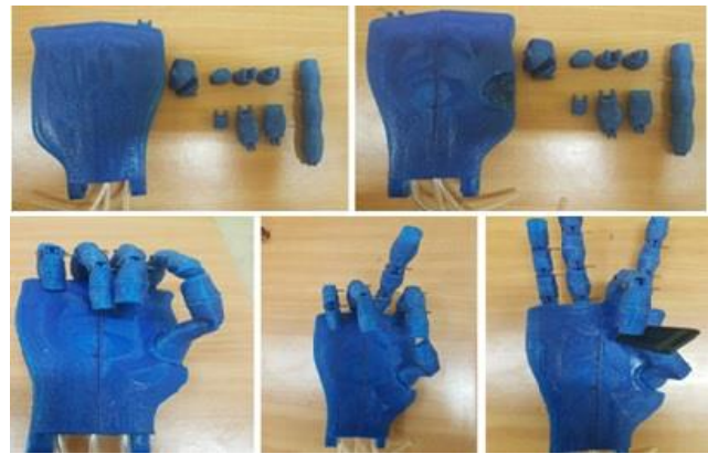
Fig. 16. Printed parts and various gripping functions [16].
